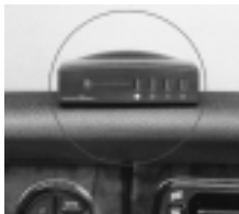
RECEIVER ATTACHED TO SURFACE WITH VELCRO® STRIPS
